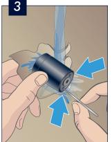
Clean frother with warm running water and use a needle to clean the two holes.
